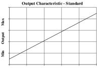
Retracted Linear Displacement Extended
