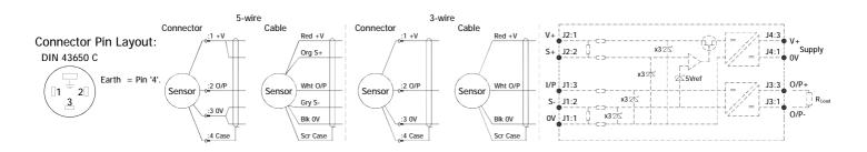
Approval only applies to specified ambient temperature range and atmospheric conditions in the range: 0.80 to 1.10 Bar, oxygen  $\leq$  21%. The G106 is available with the following connections:-
